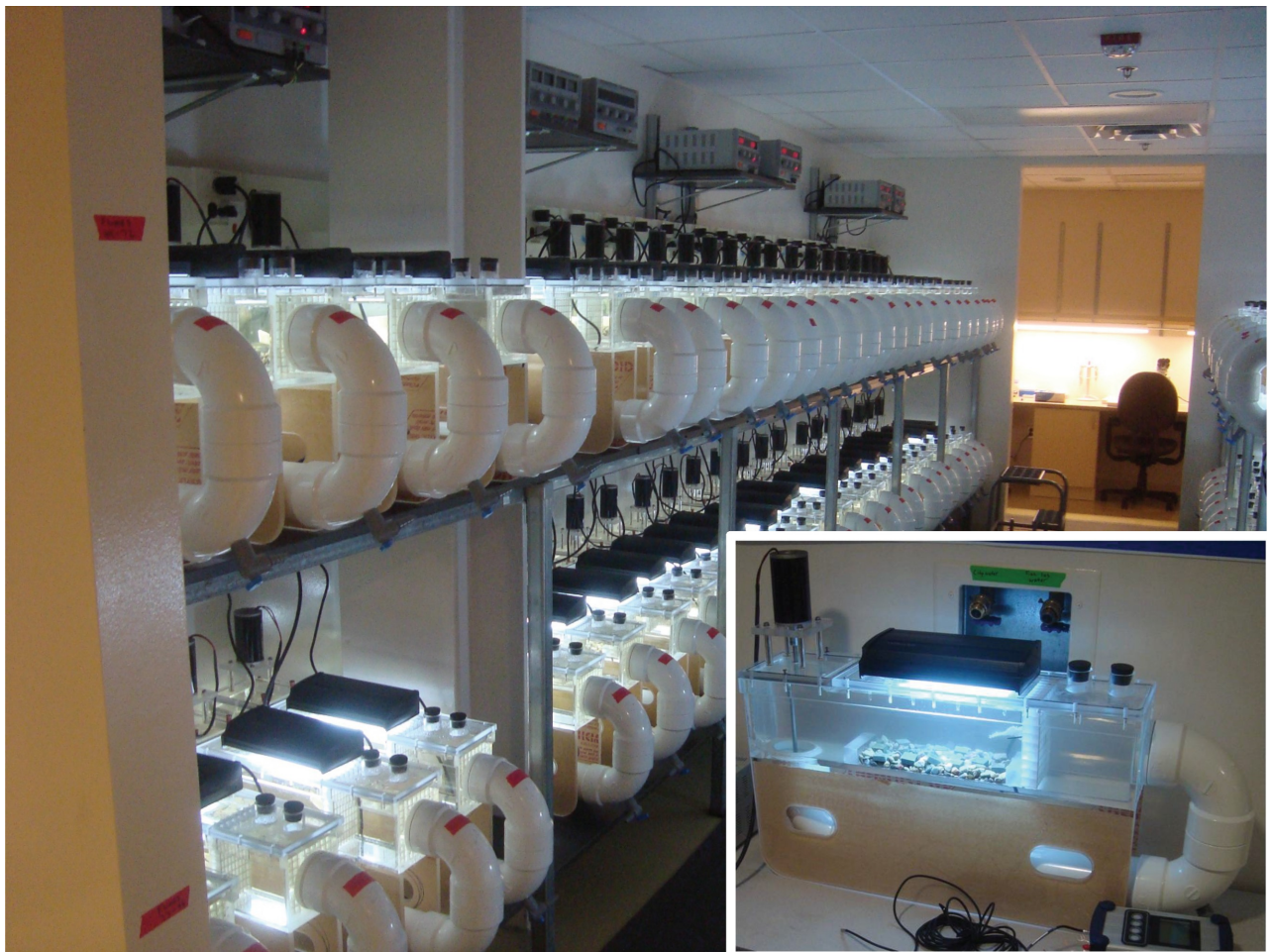
Fig 1. Images of the re-circulating mesocosms shown in use during the experiment. Inset: Close-up of one re-circulating flume including the DC motor at top left, fluorescent light on top, and pea gravel and tiles in the flume.
